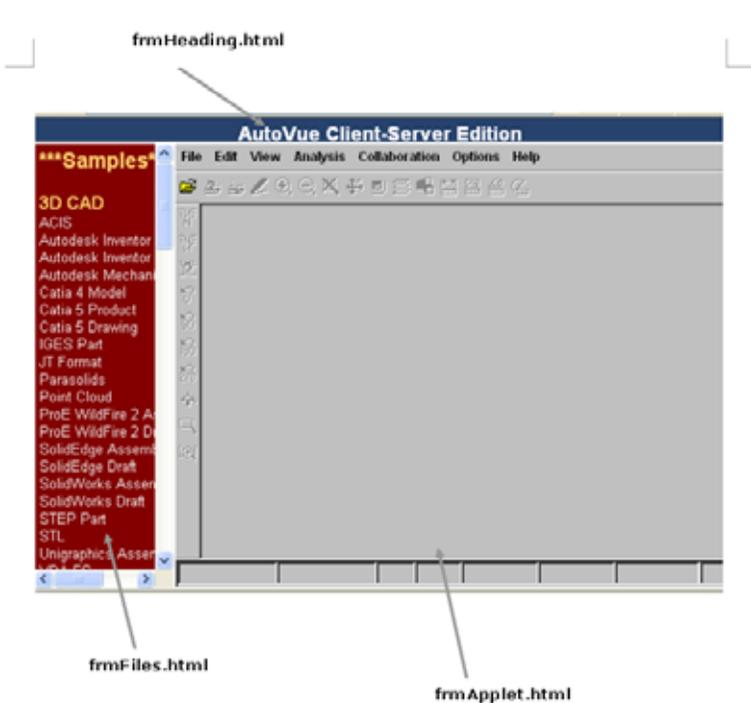
The HTML code responsible for the applet generation is held in `frmApplet.html`. The code in `frmApplet.html` holds the `<APPLET>` tag with the customizable parameters and provides a JavaScript method called `setFile` to allow `frmFiles.html` to dynamically change the file displayed in the applet, see [Scripting the Applet](#).
