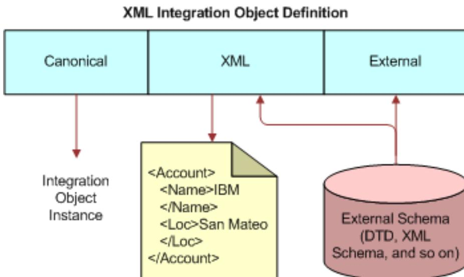
The integration object schema in the Siebel Repository is composed of the three data sections shown in the following table.
