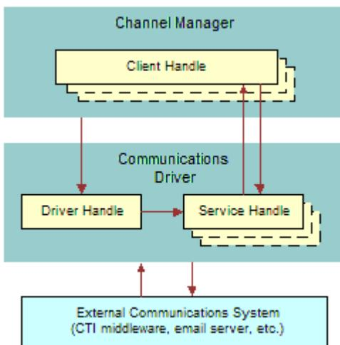
The channel manager initializes the implementation object for the driver handle, which in turn initializes the implementation object for the service handle.
