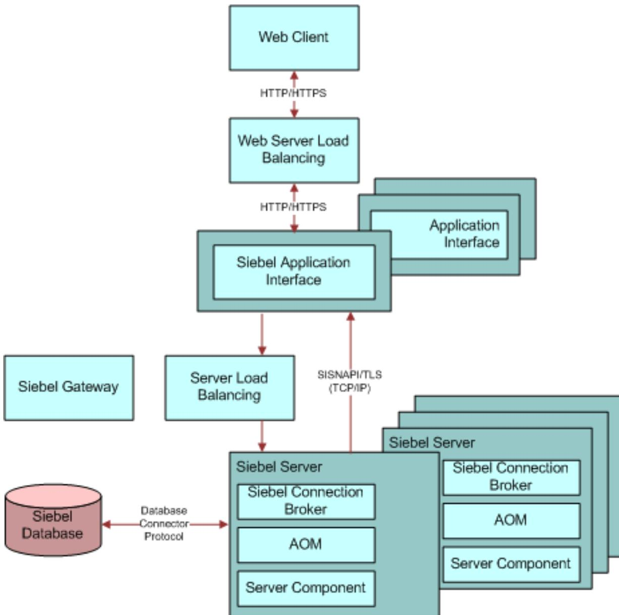
A typical Siebel client request flows from the user's Siebel Web Client through the system components for Siebel CRM applications and back again, according to the following general flow:
