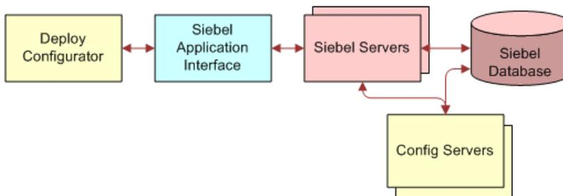
In many cases, the option of deploying Siebel Product Configurator on a different application server computer might result in a much better use of resources due to pooling effects. Considering the example examined and sized from the preceding topic, the result was a sizing of one factory and one worker to be cached for each Application Object Manager on each server. The implications of this approach across the whole enterprise are as follows:
