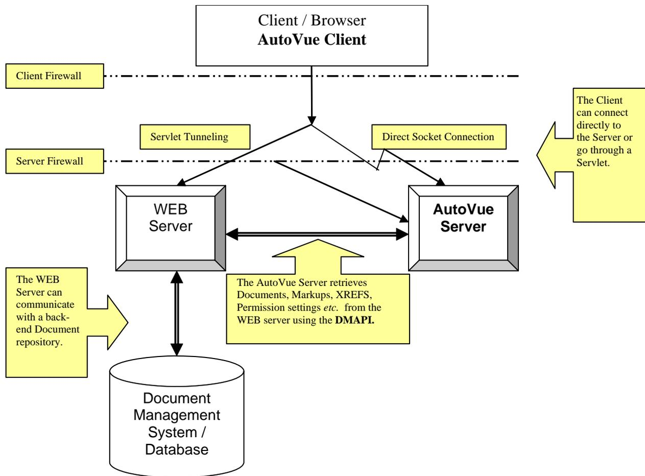
The above diagram illustrates the fundamental architecture of the AutoVue Web Version / Document Management environment. In real-world deployments, multiple AutoVue Servers may be present, and the client may be communicating with the servers through a client proxy. These facilities can provide performance and security enhancements but do not affect the implementation of the DMAPI.
