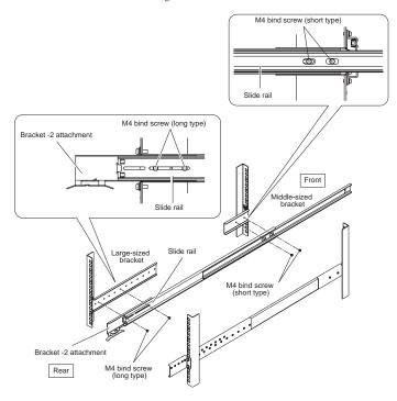
\*1: To secure the middle-sized bracket to the slide rail, use the center of the oval hole on the rail. \*2: When multiple screw holes are available on the large-sized bracket, use the holes that are nearest to and farthest from the rear column.
