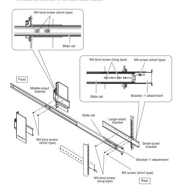
\*1: To secure the middle-sized bracket to the slide rail, use the center of the oval hole on the rail. \*2: When multiple screw holes are available on the large-sized bracket, use the holes that are nearest to and farthest from the rear column.
