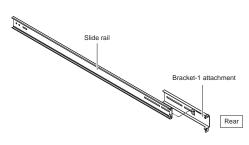
In the same manner, attach the bracket-2 to the end of the left slide rail, as viewed from the rear of the rack.
