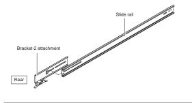
Note - The left and right brackets are different in shape. Each bracket must be installed in its proper position
