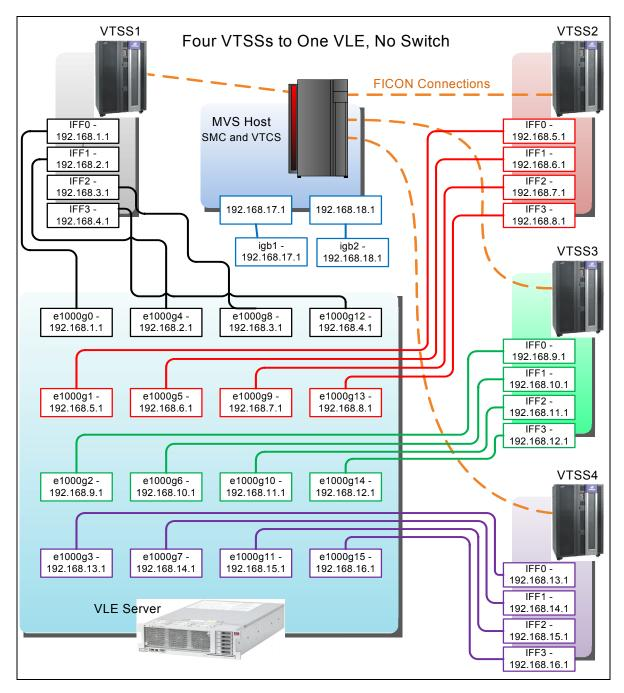
FIGURE A-8 Example 2: Four VTSSs Connected to One VLE
