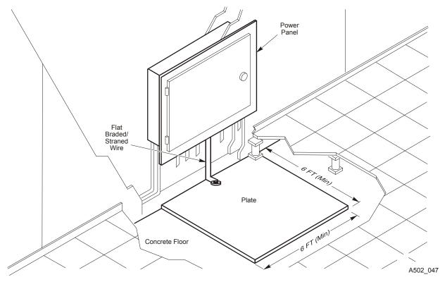
FIGURE 4-2 Transient Electrical Grounding Plate
