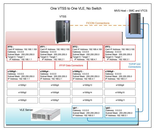
FIGURE A-7 Example 1: One VTSS Connected to One VLE
