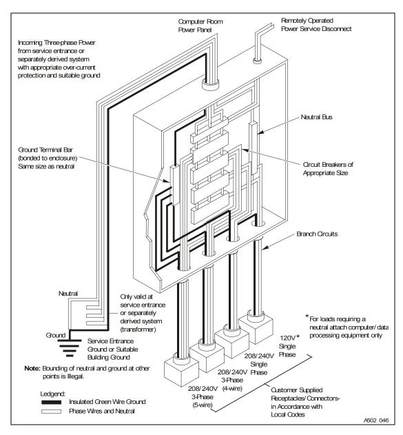
FIGURE 4-1 Site Electrical Power Distribution System
