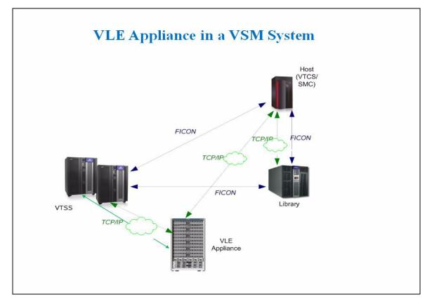
FIGURE 1-1 VLE Appliance in a VSM System
