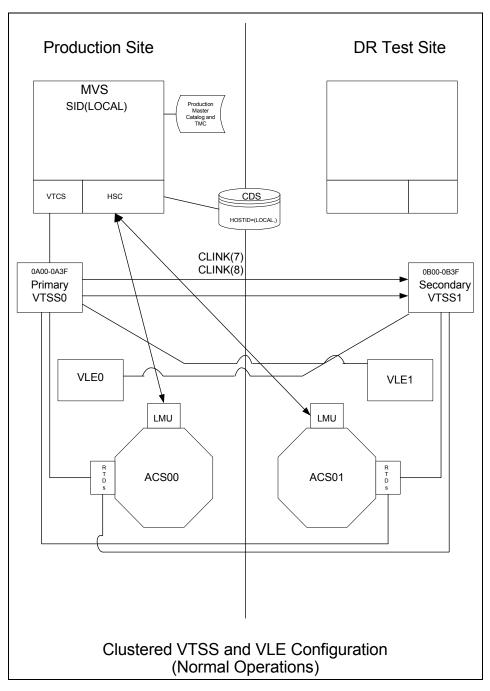
**FIGURE 3-7** Primary/Secondary Clustered VTSS and VLE Configuration - Normal Operations
