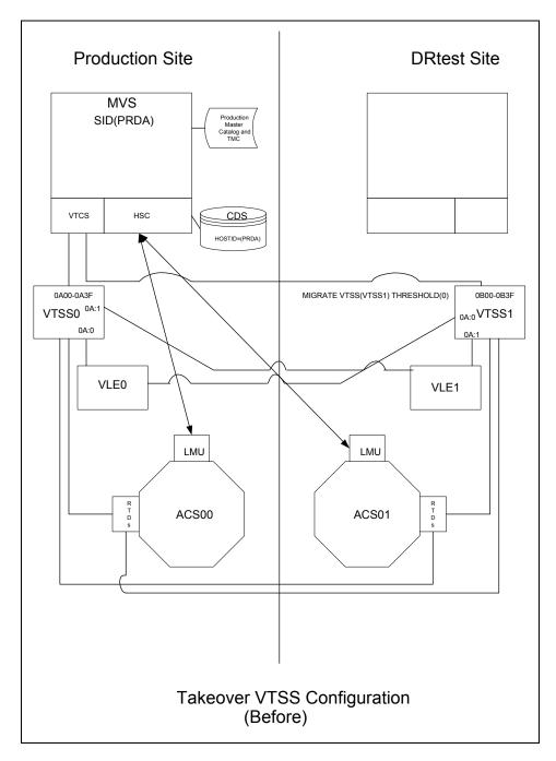
FIGURE 3-3 VLE and ACS Configuration - Before Running the DRTEST Utility
