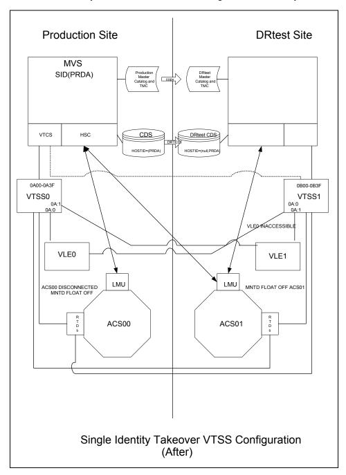
FIGURE 3-4 shows the system for Scenario 1 after running the DRTEST utility.
