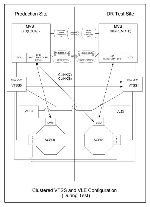
What if you wanted to use the DR Test Site for testing? FIGURE 3-8 shows the system for Scenario 3 during the DR test.
