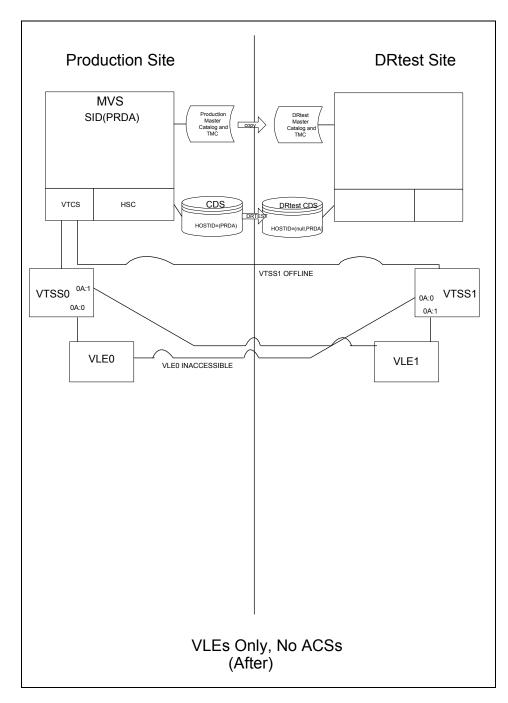
FIGURE 3-6 shows the system for Scenario 2 after running the DRTEST utility.
