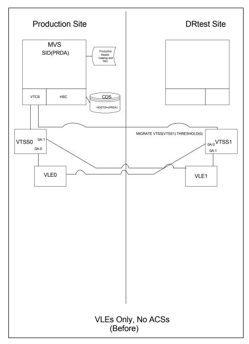
FIGURE 3-5 VLE Only Configuration - Before Running the DRTEST Utility
