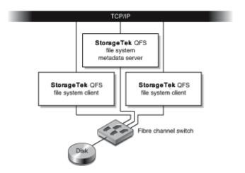
Figure of a StorageTek QFS shared file system on multiple hosts.
