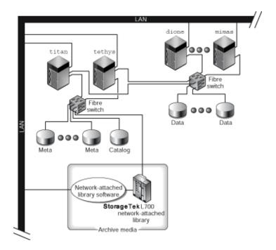
Figure of a shared StorageTek ASM-QFS environment. Shows hosts titan, tethys, dione, and mimas connected to a LAN.
