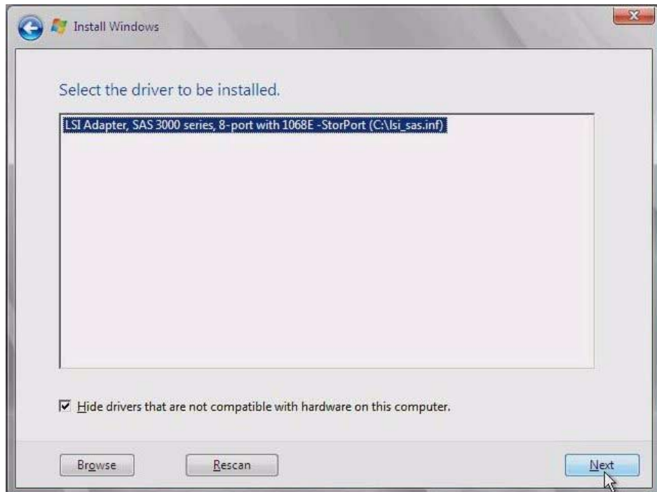
FIGURE 6-6 Select the Driver to be Installed Screen
