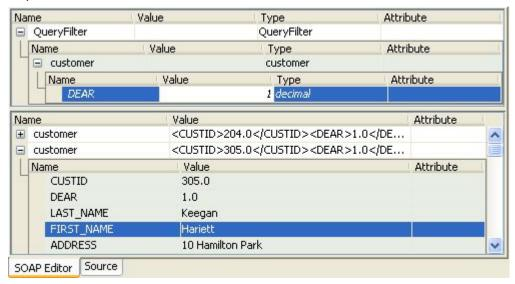
The upper part of the editor shows the hierarchical structure of the query, the lower part shows the structure of the response. This arrangement can be changed using the  $\square$  **Switch Panel Position** button.
