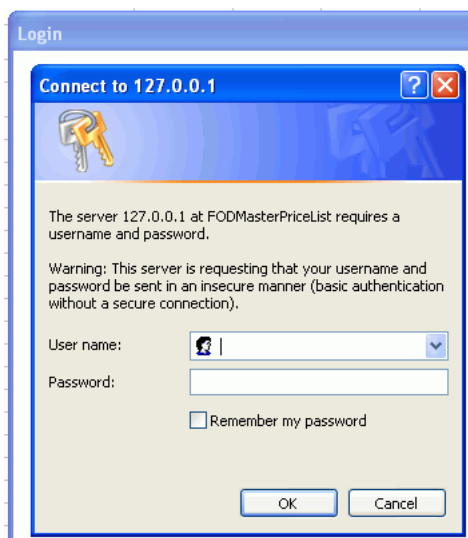
Figure 11-1 Dialog Box That Appears When a Fusion Web Application Uses Basic Authentication
