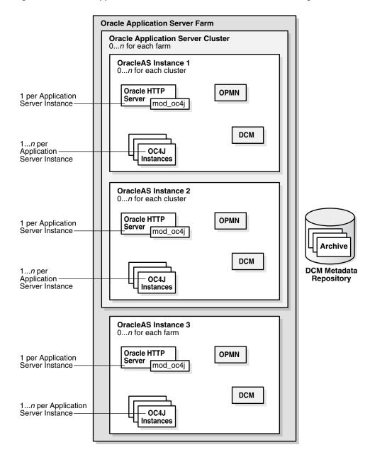
Figure 2–1 Oracle Application Server Farm, Instance, and Cluster Configuration
