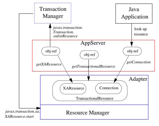
In this usage scenario, the XAResource interface is transparent to the application program, and the Connection interface is transparent to the transaction manager. The application server is the only party that holds a reference to some TransactionalResource object.
