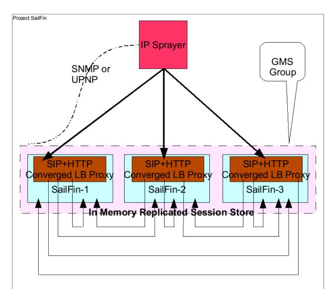
It is very likely that the load balancer tier is fronted by a hardware IP level load balancer (or IP sprayer).
