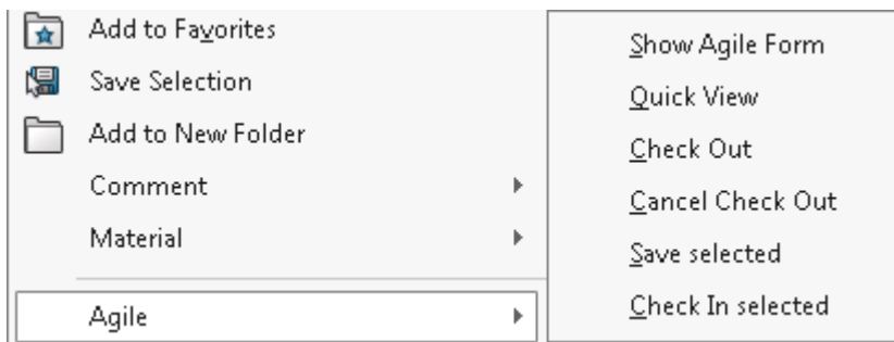
Figure 2: An example of the CAD context menu directly embedded into CAD.
