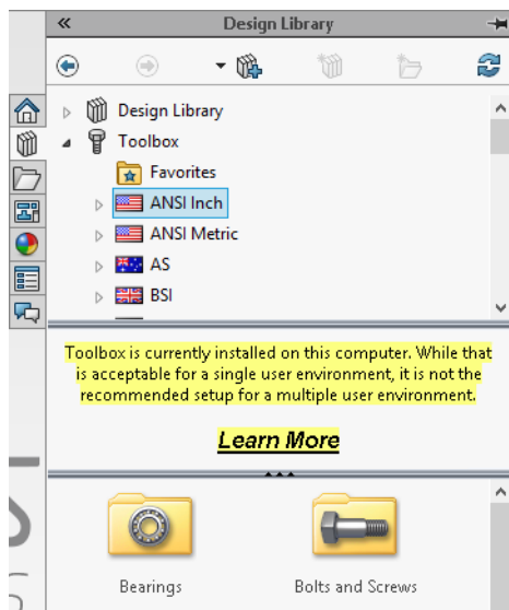
Figure 51: Design Library workspace in SOLIDWORKS
