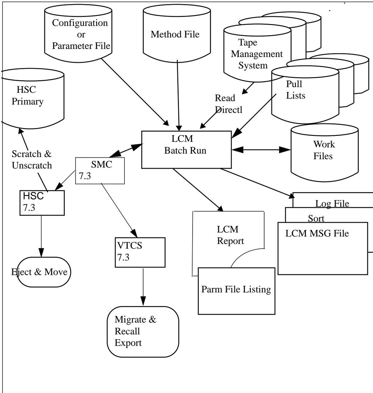
FIGURE 1-1 LCM Processing
