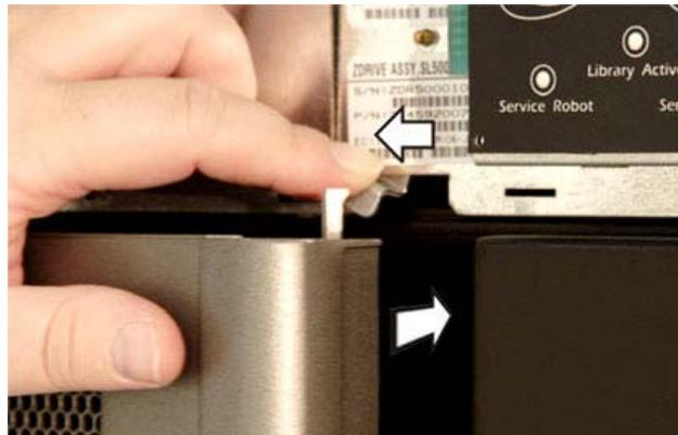
3. While still holding the door shut, release the robotics park lever.
