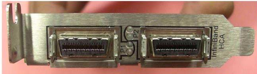
FIGURE B-10 Assembled Short Bracket View
