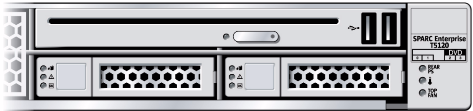
FIGURE: DVD/USB Module in a Sun SPARC Enterprise T5120 Server
