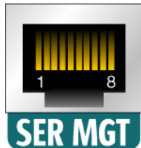
FIGURE A-1 Serial Management Connector Diagram
