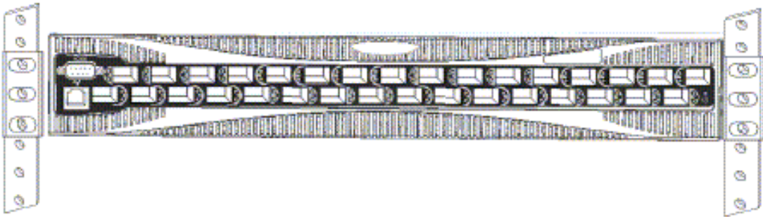
FIGURE 3-1 SilkWorm 3900 Switch Installed With Additional 0.5 RU Above L-Brackets
