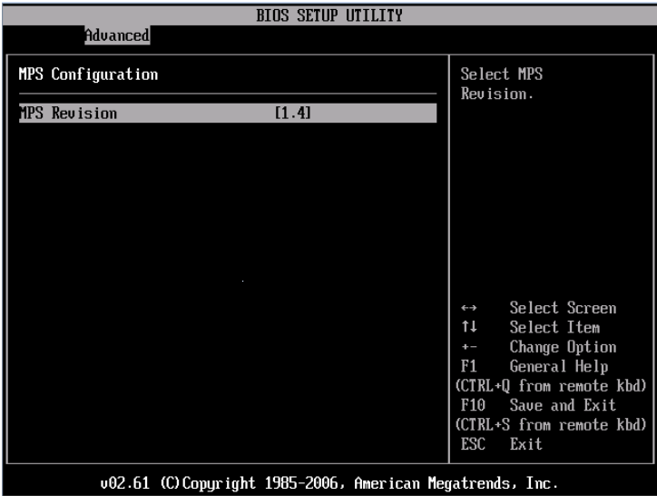
FIGURE A-17 BIOS Setup Utility: Advanced- MPS Configuration
