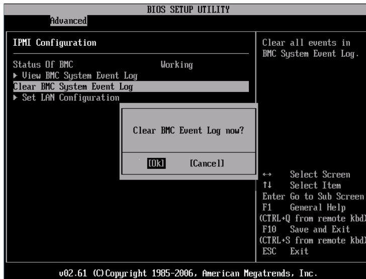
FIGURE A-14 BIOS Setup Utility: Advanced - IPMI - Clear BMC System Event Log
