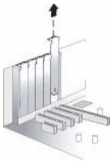
FIGURE 2-3 Remove Slot Cover from Expansion Slot
