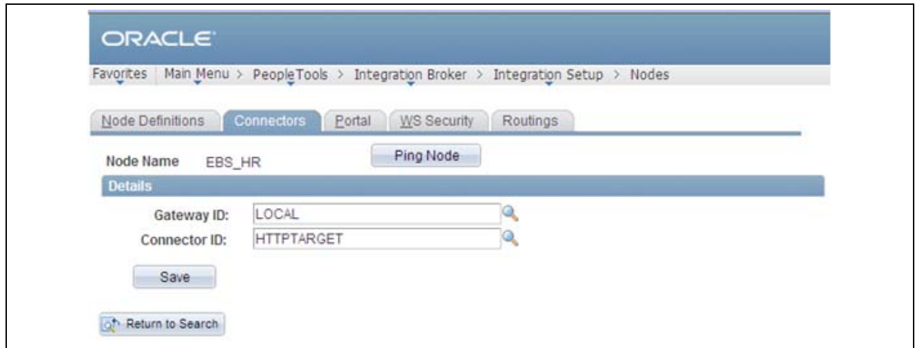
Connectors tab with EBS_HR node connector parameters
