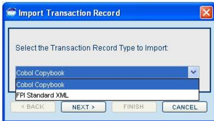
The FPI automatically parses the record transaction type and stores its associated properties and structure in the workspace. Individual groups and fields of the copybook are displayed as new nodes, listed below the transaction record node. Each field has many attributes associated with it, which were automatically parsed from the copybook when it gets imported. Some additional properties are added, which can be modified by the user (such as error conditions).
