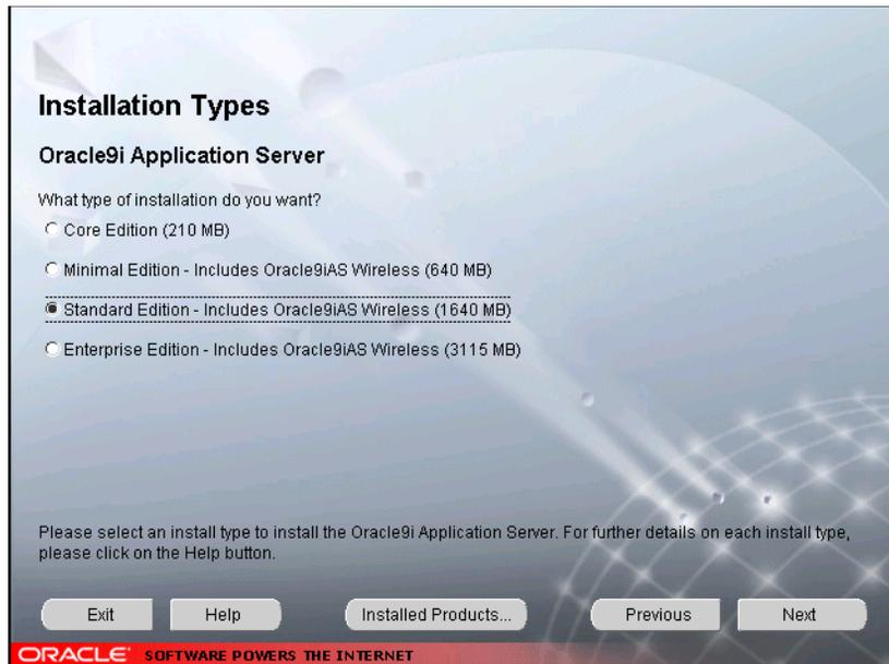
The Installation Types screen allows you to select the Oracle9i Application Server installation option that you are licensed to use.
