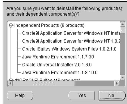
The Confirmation screen lists all the components selected for deinstallation in the previous step. Scroll down the screen to verify selected components.
