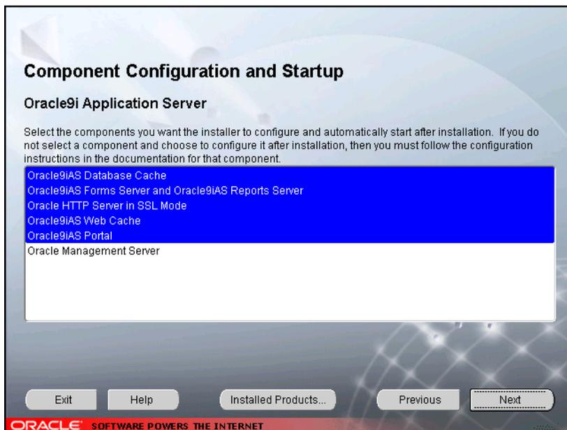
The Component Configuration and Startup screen allows you to select the components that you want the installer to configure and start after installation. This screen offers two configuration options:
