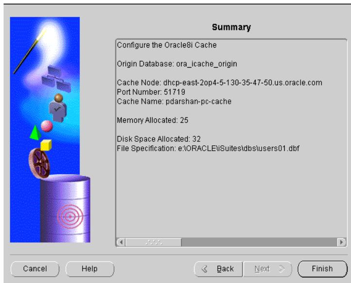
The Summary screen provides information about the origin database, cache node, port number, cache name, memory, disk space allocated and file specification.
