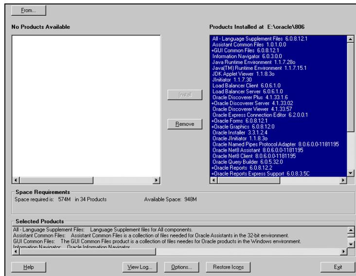
The Software Asset Manager allows you to deinstall components. Be sure to scroll down to select all installed components. When you click **Remove**, a dialog appears asking you if you want to remove the selected components. Click **Yes**. When all the components are deinstalled, quit the installer by clicking **Exit**.
