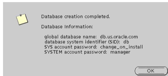
The Database Information screen displays database information such as global database name, database SID, SYS account password, and SYSTEM account password. Make a note of this information and click **OK**. You have completed the database creation process.
