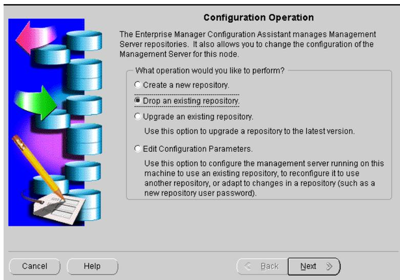
Configuration Operation Screen allows you to create, drop, or upgrade a repository. It also enables you to edit your configuration parameters.
