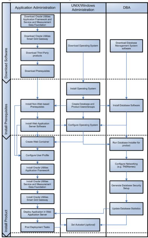
The following diagram provides an overview of the steps that need to be taken to install and configure Oracle Utilities Smart Grid Gateway:
