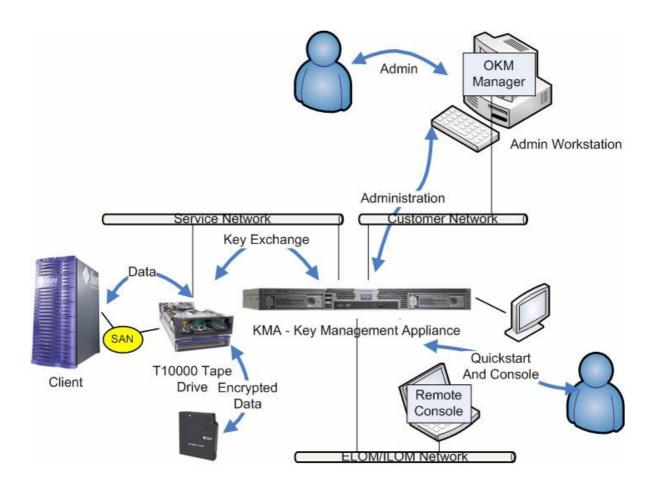
Figure 1-1. Connections to the KMA
