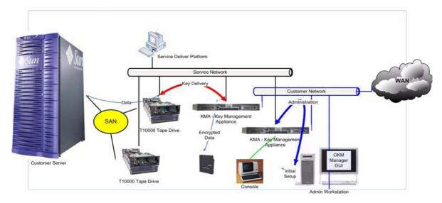
Figure 1-2. Typical Deployment of OKM Solution
