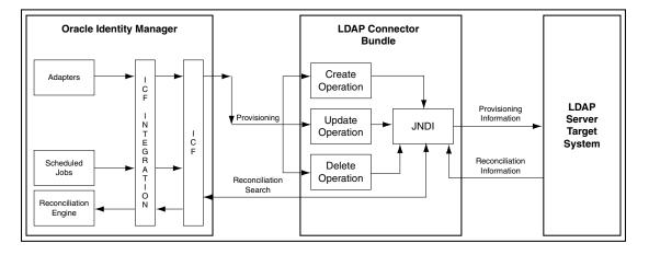
The OID connector uses JNDI to access the target system.
