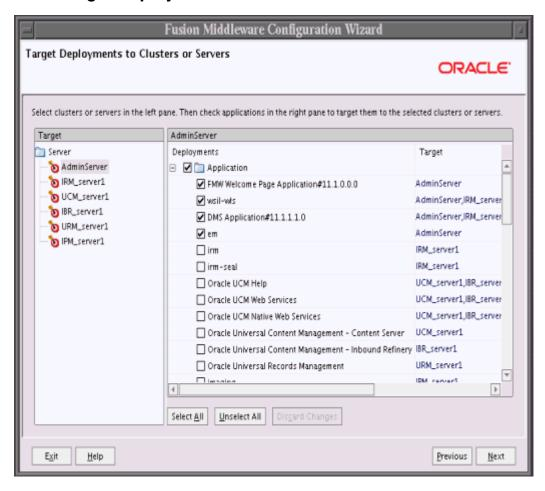
Use this screen to target your deployments to Managed Servers or to clusters of Managed Servers. Doing so enables Oracle WebLogic Server to serve the deployments to clients.
