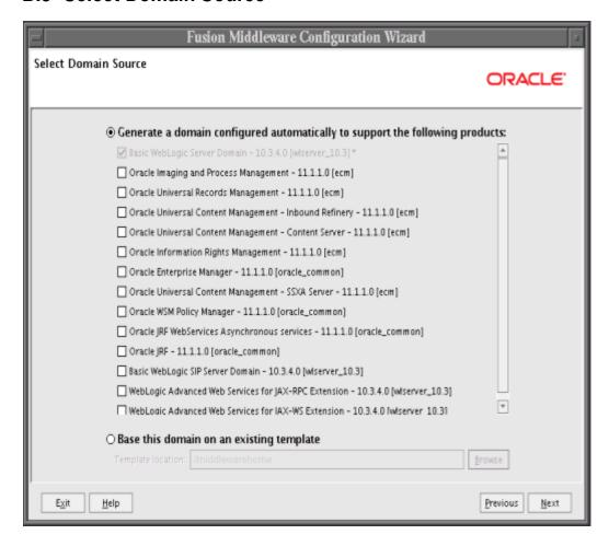
Select the source from which to create a new Oracle WebLogic Server domain. Select Generate a domain configured automatically to support the following products to create your domain to support selected products, and then select the products.
