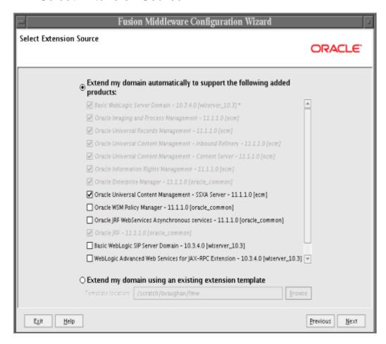
Select the source from which to extend an existing Oracle WebLogic Server domain. Select Extend my domain automatically to support the following added products, and then select the products.
