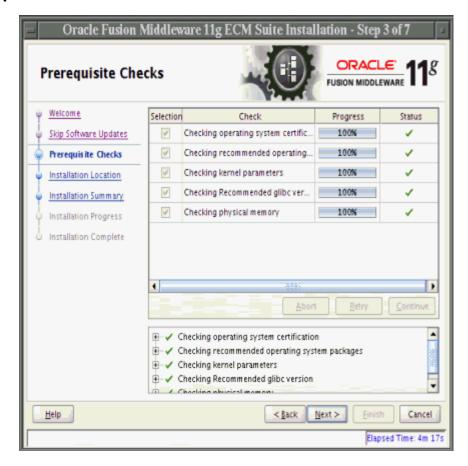
This screen shows the prerequisite checks for a UNIX operating system. Only three checks are performed for a Windows operating system:
