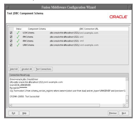
Use this screen to test JDBC connections to application schemas.
