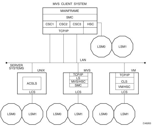
Figure 1. MVS/CSC-to-LCS Configuration
