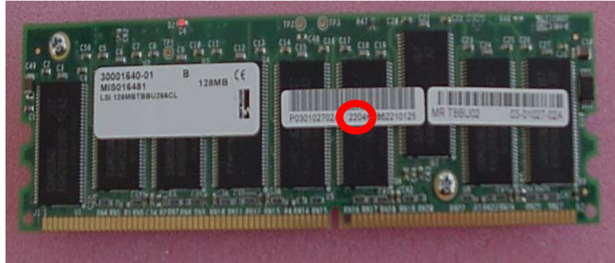
FIGURE 2 Transportable Battery Backup Unit With Date Code Circled
