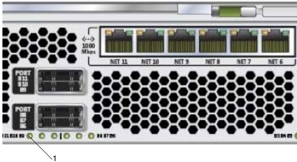
FIGURE 1-2 Sun Blade 6048 Switched InfiniBand Express NEM Port LED Indicators
