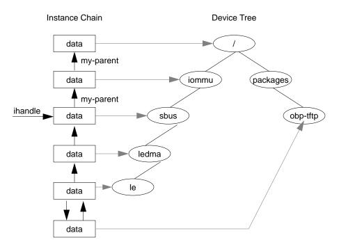
Figure 4-2 An Instance Chain for /iommu/sbus/ledma/le with obptftp Support
