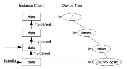
Figure 4-1 An Instance Chain for /iommu/sbus/SUNW,cgsix
