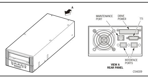
The T9840B/C/D rear panel has a Maintenance Port (standard RJ45 receptacle) for Service Delivery Platform (SDP) and/or Customer Service Engineering (CSE) interface.
