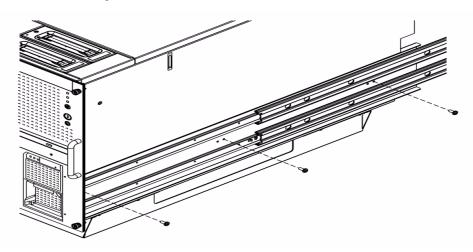
6. Remove the plinth from the bottom of the server (FIGURE 6-9).
