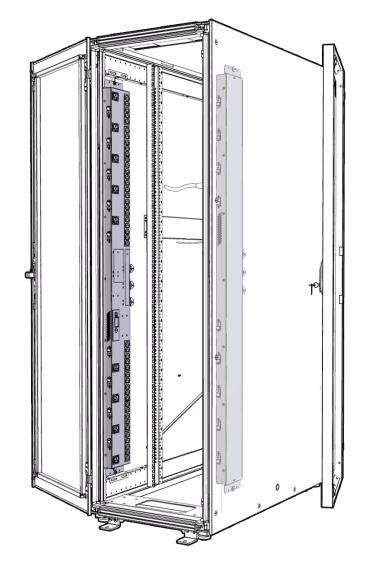
FIGURE 2-1 Sun Rack II With Two PDUs
