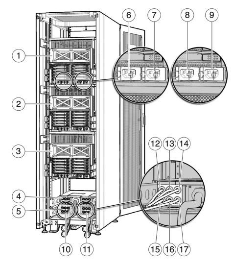
FIGURE 7-1 Sun Rack 1000 With Three M5000 Servers and Two MPS
