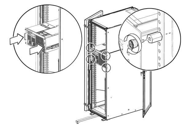
FIGURE 4-12 Example of Spacers Aligned With Captive Screws
