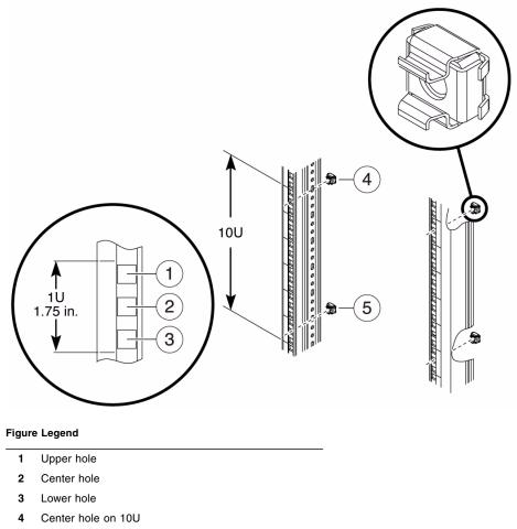
FIGURE 6-3 Cage Nut Hole Locations for the M5000 Server
