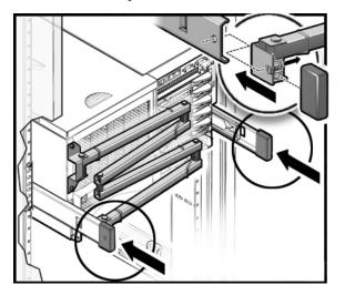
2. Connect the power cables to the rear of the server and secure them with the cable retention clamps.
