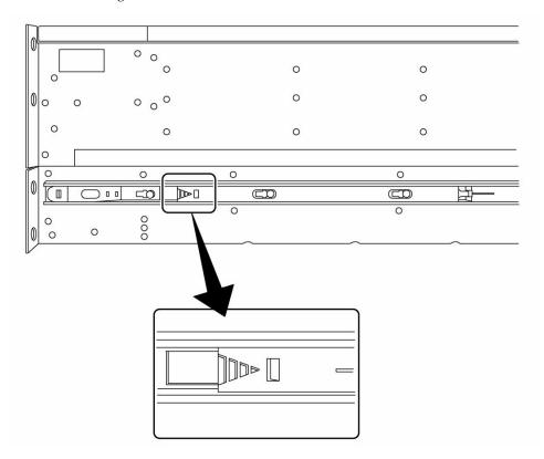
FIGURE 4-11 Locking Mechanism on the M4000 Slide Rail
