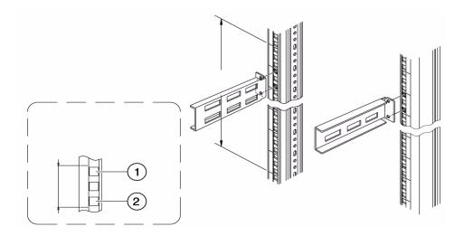
4. Insert the hook and loop straps in the desired slots of the bracket to hold back cables.
