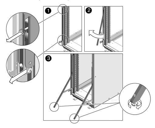
FIGURE B-2 Extending the Anti-Tilt Legs
