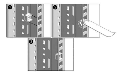
FIGURE A-1 Inserting Cage Nuts in Square Holes Using the Insertion Tool
