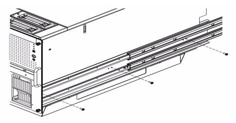
8. Remove the plinth from the bottom of the server (FIGURE 6-14).
