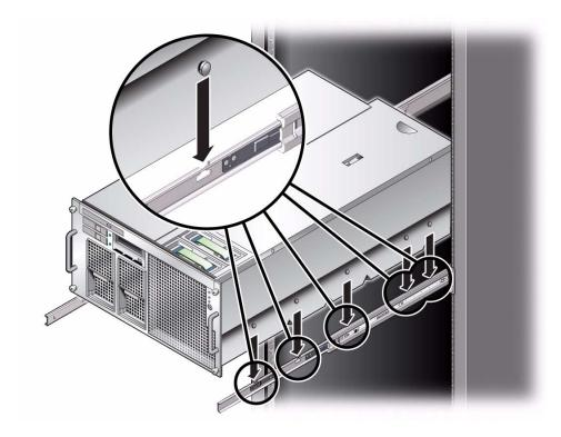
FIGURE 4-9 Aligning Server Pins With Version 2 Slide Rail Keyholes
