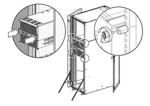
FIGURE 6-16 Example of Spacers Aligned With Captive Screws
