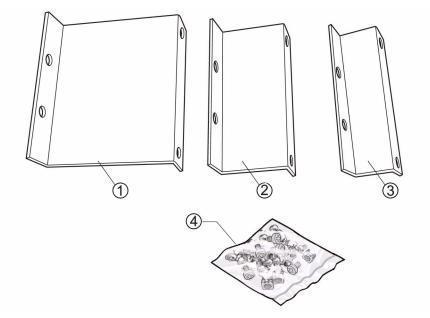
FIGURE 6-2 M5000 Shipping Bracket Kit Contents
