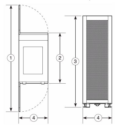
FIGURE 1-3 Sun Rack 900 With Cabinet Extender Top and Front Dimensions
