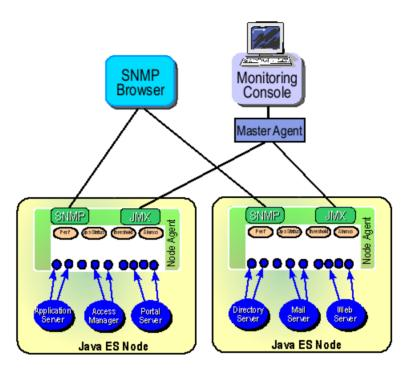
FIGURE 1-2 Diagram of the Overall Monitoring Architecture
