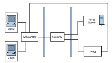
FIGURE 4-19 Secure Remote Access Gateway with External Accelerator
