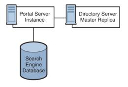
FIGURE 4-4 Portal Server Building Module Architecture
