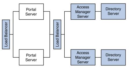
Figure 4–8 illustrates Access Manager and Portal Server residing on separate nodes.
