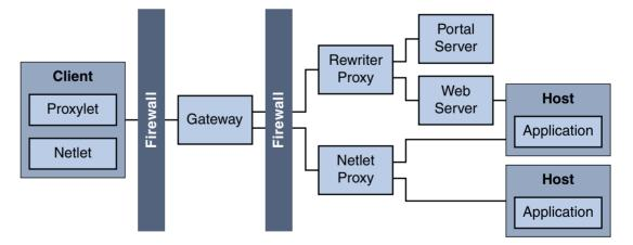
FIGURE 4–3 Secure Remote Access Deployment
