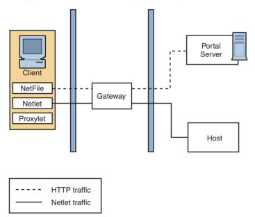
FIGURE 4–12 Basic Secure Remote Access Configuration
