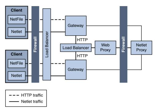
FIGURE 4–18 Two Gateways and Netlet Proxy
