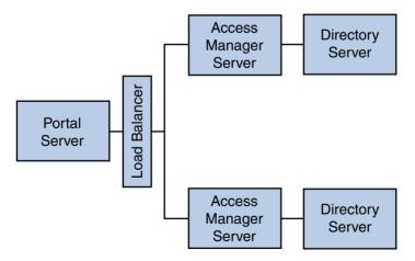
FIGURE 4-11 Load Balancing two Access Managers
