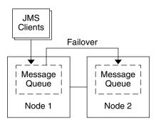
FIGURE 1 Two-Node Cluster with Failover Data Service Configuration
