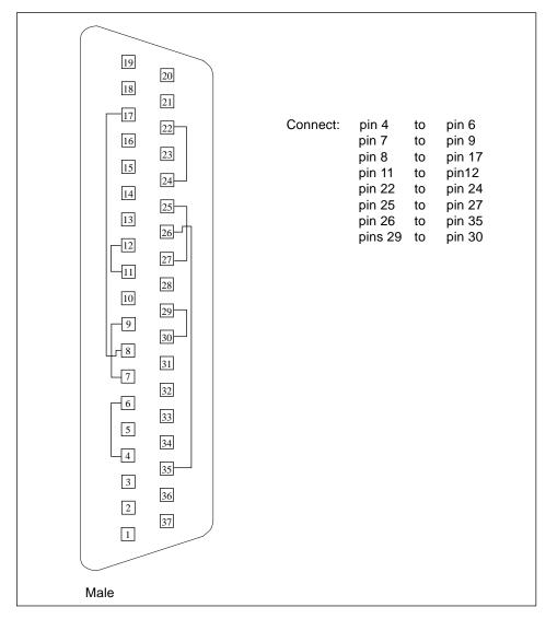
FIGURE A-10 37-Pin RS-449 Loopback Plug
