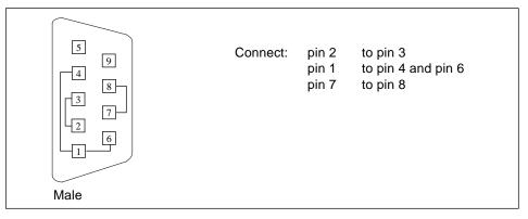
FIGURE A-11 9-Pin Male Single-port Loopback Plug
