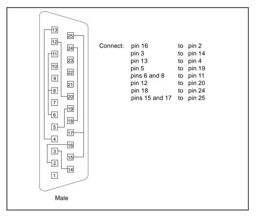
FIGURE A-5 Port A-to-Port B Loopback Plug
