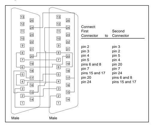
FIGURE A-2 25-pin RS-232 Port-to-Port Loopback Cable
