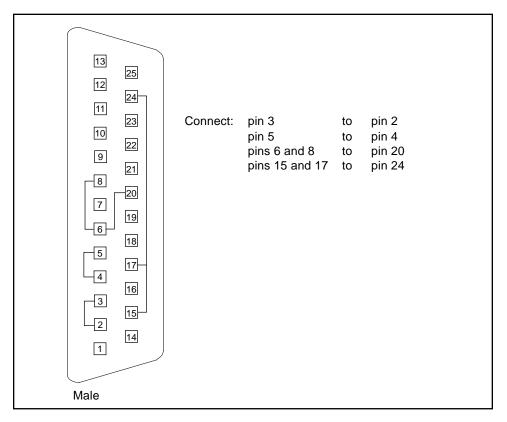
FIGURE A-1 25-pin RS-232 Loopback Plug
