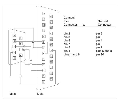
FIGURE A-13 9-Pin to 25-Pin Port-to-Port Loopback Cable
