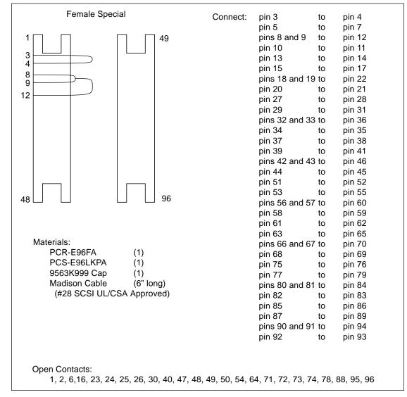
FIGURE A-8 96-Pin Female Special Loopback Connector
