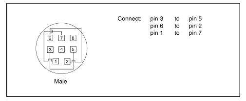
FIGURE A-4 8-Pin Loopback Plug
