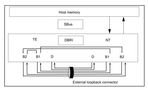
FIGURE 16-4 isdntest Data Path Subtest
