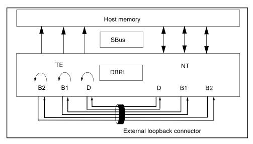
FIGURE 16-2 isdntest Remote Loopback Subtest
