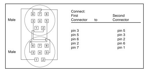
FIGURE A-3 8-Pin to 8-Pin Loopback Cable
