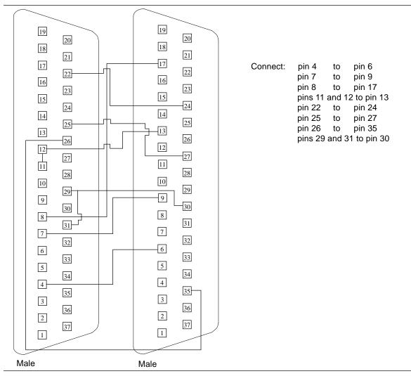
Use these wiring instructions for a loopback cable for two 37-pin RS-449 synchronous ports (see FIGURE A-9).
