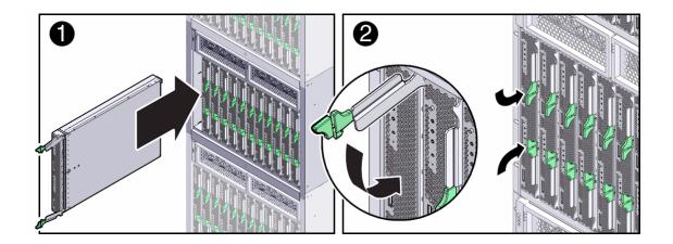
9. Lock the server module into the chassis. Rotate the top ejector down while rotating the bottom ejector up until they both latch into place.
