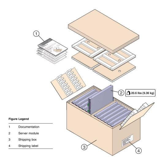
**FIGURE 1-2** Shipping Box Contents (Single Blade)
