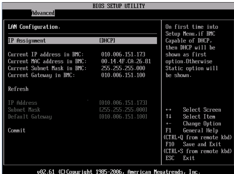
FIGURE A-15 BIOS Setup Utility: Advanced - IPMI - LAN Configuration -IP Assignment
