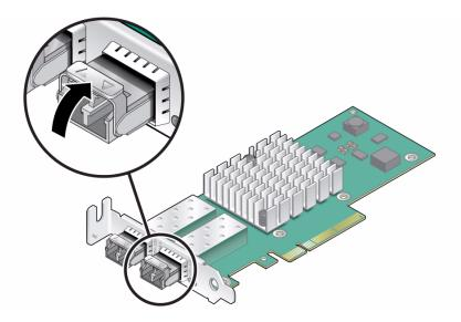
5. Repeat Step 1 through Step 4 to install the second optical transceiver.
