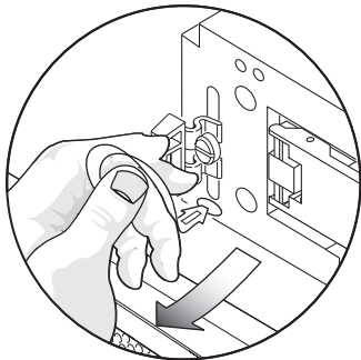
FIGURE 5-10 Pulling the Head of the Tether out of the Array
