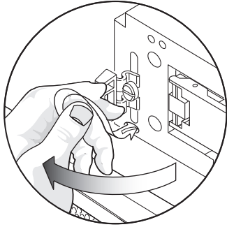
FIGURE 5-8 Pushing the Tether to One Side Until its Head Emerges
