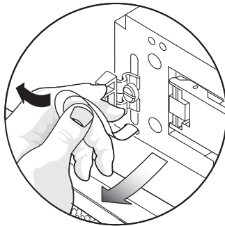
FIGURE 5-7 Pulling a Tether Until It Stops
