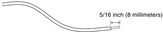
FIGURE 2-6 Stripping the Insulation From the Wire
