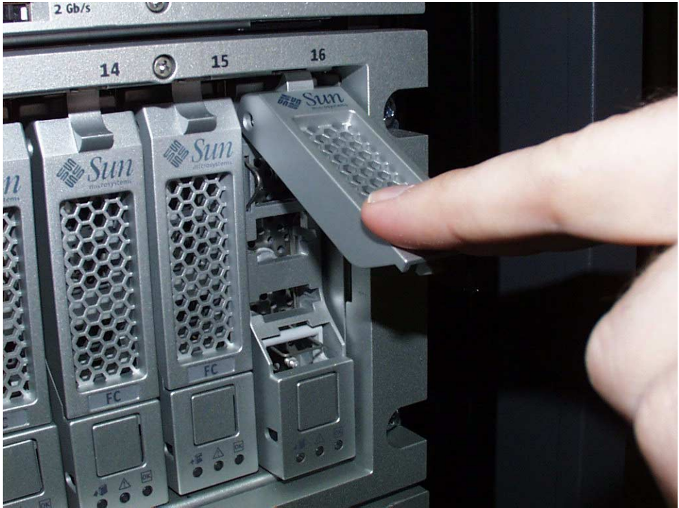
FIGURE B-1 Inserting a Disk Drive
