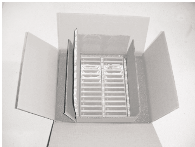
Figure 14. Double-boxing tape cartridges for shipping
