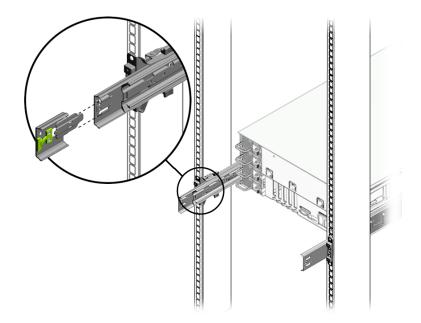
4 Insert the right inner latch (numbered 6 in the CMA illustration) into the right rear slide rail. The inner latch does not have the green insert.
