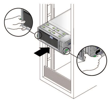
4 With two hands, slide the green plastic tabs toward you to release the lock and push the server all the way into the rack.
