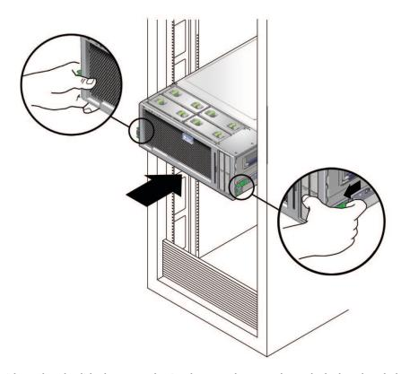
5 With two hands, slide the green plastic tabs toward you to release the lock and push the server all the way into the rack.
