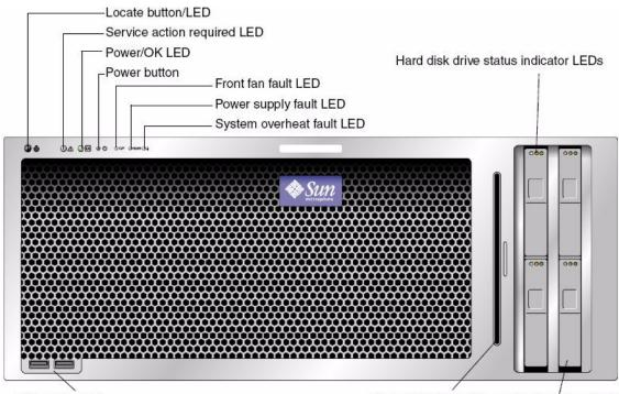
FIGURE 1-1 Sun Fire X4600/X4600 M2 Servers Front Panel Features
