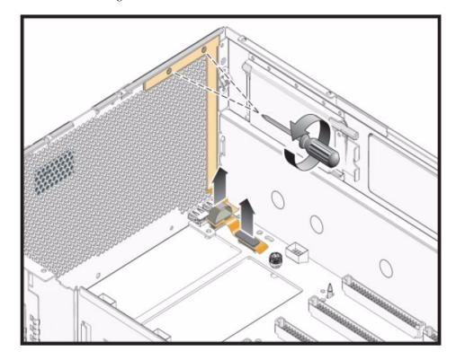
FIGURE 3-11 Removing the Front Panel Indicator Board
