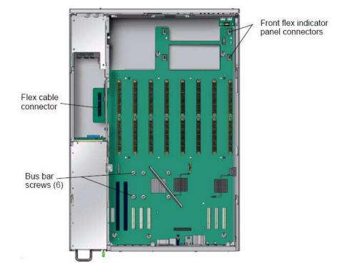
e. Slide the small metal door in the chassis midwall near the flex-cable connector upward to provide clearance for the power tab of the motherboard. See FIGURE 3-20.
