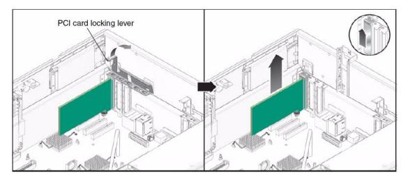
FIGURE 3-22 Opening the PCI Card Locking Lever and Removing the PCI Card
