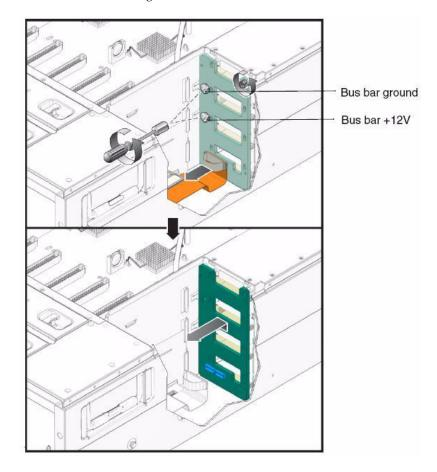
FIGURE 3-25 Disconnecting the Power Distribution Board From the Chassis
