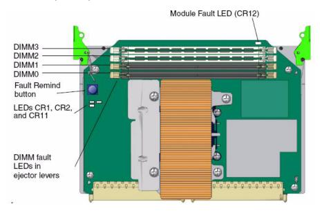
FIGURE F-2 Physical Layout of Sun Fire X4600 M2 4-DIMM CPU M
