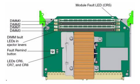
FIGURE F-1 Physical Layout of Sun Fire X4600 CPU Module
