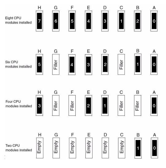
**Note** – In six-module and four-module configurations, unused CPU slots must contain filler modules. In two-module configurations, unused CPU slots must be left empty.
