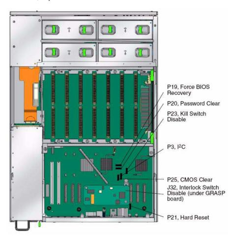
FIGURE C-6 Jumpers on the Motherboard
