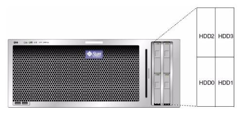
FIGURE 3-14 Sun Fire X4600/X4600 M2 Designation of Hard Disk Drives
