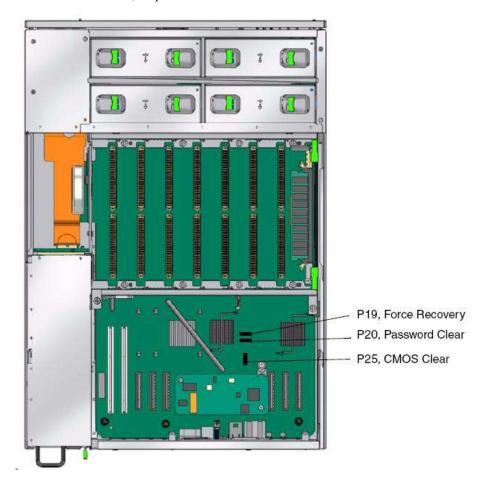
FIGURE 2-6 Location of Jumpers on the Motherboard
