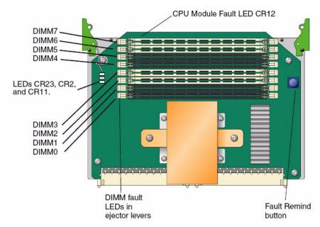
FIGURE F-3 Physical Layout of Sun Fire X4600 M2 8-DIMM CPU Module and Sun Fire X4600 M2 8-DIMM Split Plane CPU Modules
