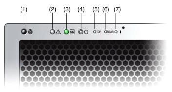
FIGURE 1-2 Sun Fire X4500 Server Front Panel Controls and Indicators
