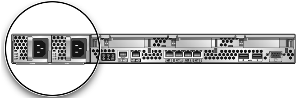
FIGURE 6-4 Rear Panel Power Supplies
